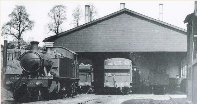
GWR engine shed like Chippenham's with a Prairie tank, 0-6-0 pannier tanks and 0-4-0 auto engines
